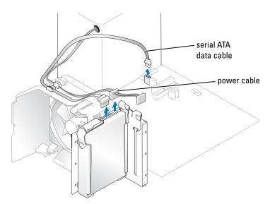
**3** Press in on the blue tabs on each side of the drive and slide the drive up and out of the computer.
